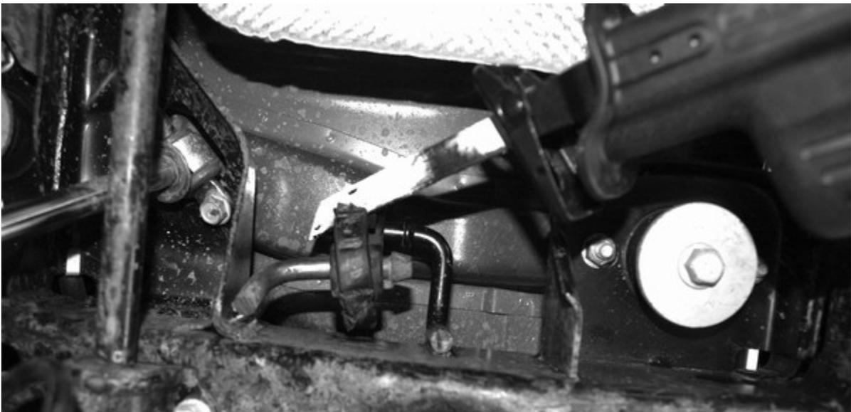
2. With some oil and a pair of channel locks, remove the drivers side muffler isolator from the exhaust hanger.
