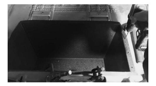
18. Tub bed-liner sealer - Generously apply a coat of bed-liner to the area that will meet the tub mount flange.
