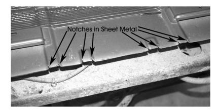
11. Hammer or Pliers - Carefully form the metal flat in order to seat properly against the top of the storage tub. (A heavy piece of steel or wood can be used to support the back side.)
