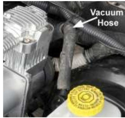
3. Loosely zip tie the vacuum hose as indicated in the previous picture, in order to assure at least  $\frac{1}{2}$ " clearance around the compressor head.
