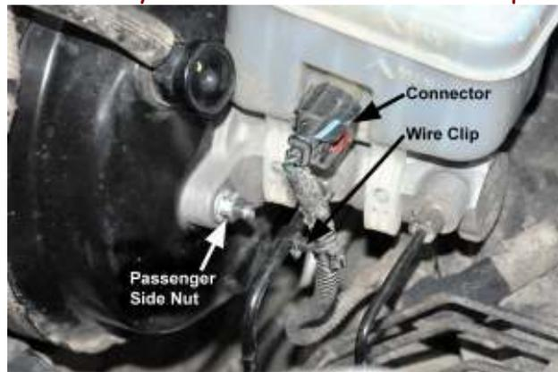
5. Remove the brake fluid sensor wire connector - With a small flat head screw driver, slide the red tab toward the passenger's side. Press the tabs and pull the connector off of the brake fluid reservoir.
