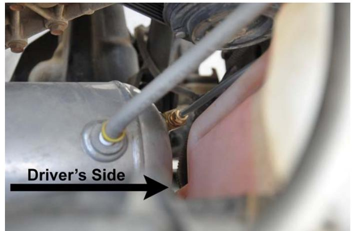
7. Place the tank into position. This is usually done from above. If using a lift with the suspension fully drooped out, the tank can be placed from below too.
