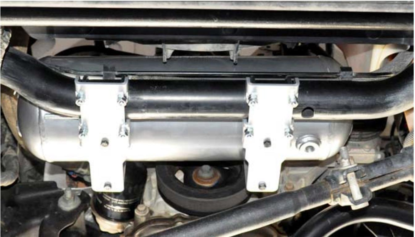
11. Using two 7/16" Wrenches Install the next 8 nuts and tighten them as jam nuts.
