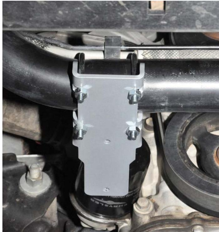
**Advisory:** If you have an automatic transmission the two transmission cooler hoses can easily be bent downward by hand, in order to allow clearance for the driver's side tank bracket.
