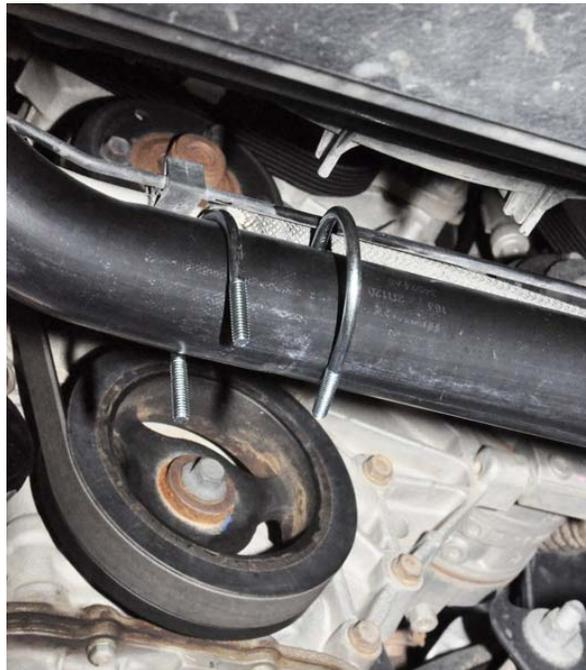
2. Place the tank mount bracket into position and firmly HAND tighten all four nuts on the passenger side.
