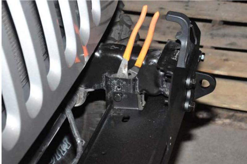
6. The factory spacers that you removed during the factory bumper removal need to be use as indicated in the following picture:
