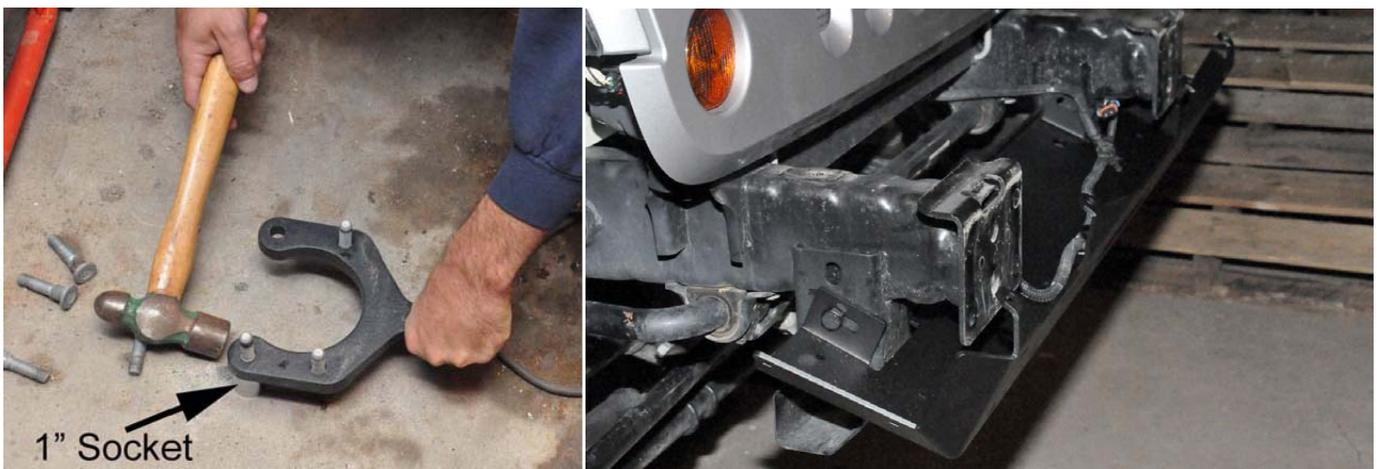
4. Supporting the bumper from below (a hydraulic jack and a block of wood are a good way to support the bumper), swing the bumper into position.
