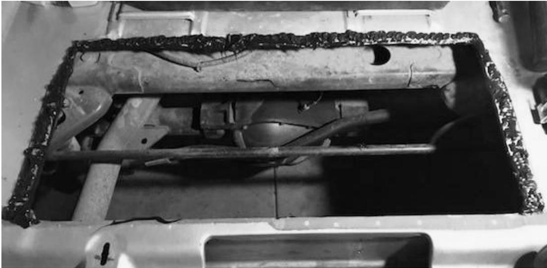
19. Tub bed-liner - Coat the bottom of the tub mount flange.
