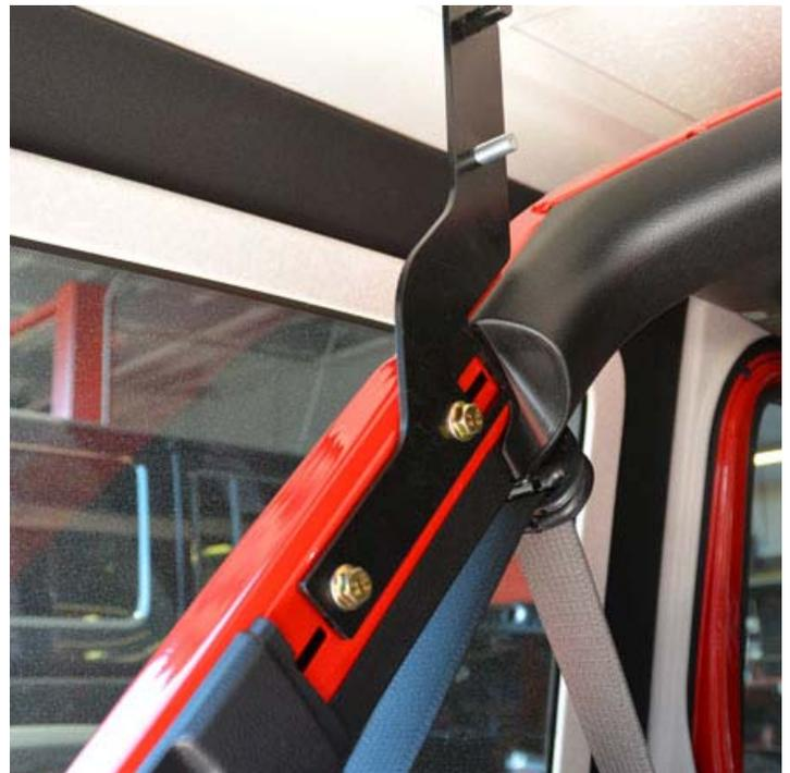
3. (2) 6mm fasteners - repeat above to attach the passenger's side bracket.
